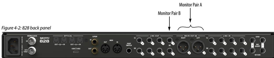
☛ Quarter-inch line outputs are not cross-coupled. Therefore, when connecting them to an unbalanced input, use a TRS plug with the ring disconnected. Not floating the negative terminal will short it to the sleeve ground and cause distortion.
