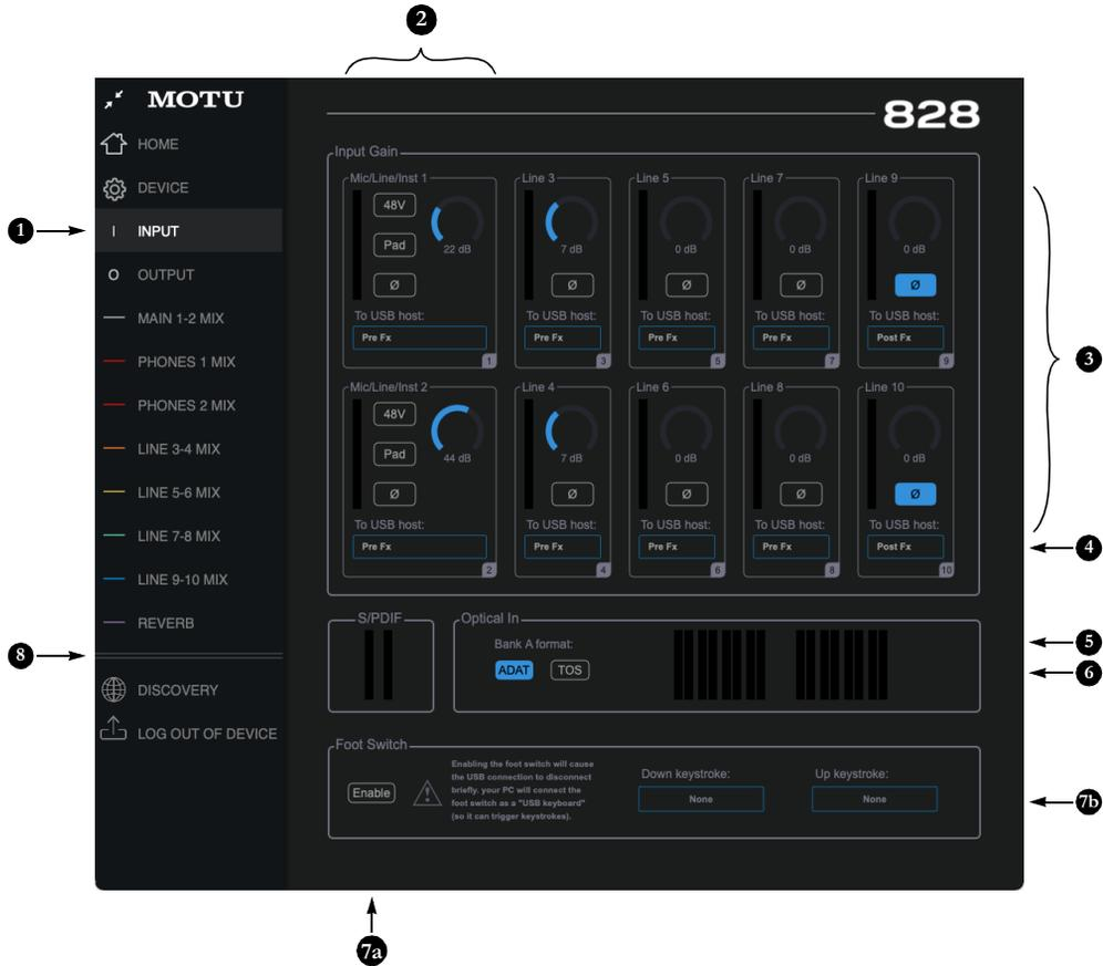
1. This is the *Input* tab, which provides access to settings for the 828 analog and digital inputs.
