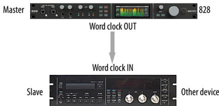
Figure 4-11: Slaving another digital audio device to the 828 via word clock. For the 828 clock source, choose *Internal* (or any source other than *Word Clock*, as daisy-chaining word clock is not recommended).
