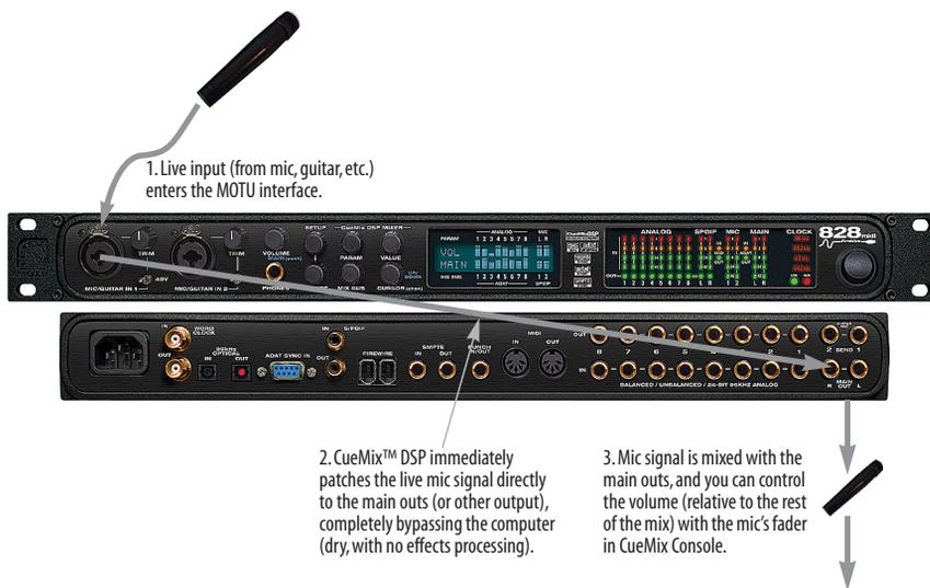
Figure 9-2: This diagram shows the signal flow when using CueMix™ DSP no-latency monitoring. Notice that this method does not allow you to process the live input with plug-ins in your audio software while it is being monitored. You can, however, add effects later — after recording the live input as a disk track. CueMix™ DSP lets you hear what you are recording with no delay and no computer-based effects.
