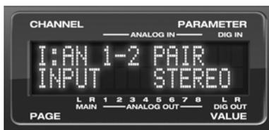
Figure 3-3: The settings for analog inputs 1 and 2 (as a pair).
