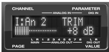
Figure 3-4: Setting the input trim for a TRS analog input pair.
