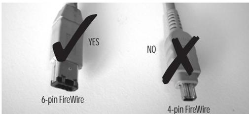
Figure 3-8: 4-pin FireWire connectors cannot be used for bus power.
