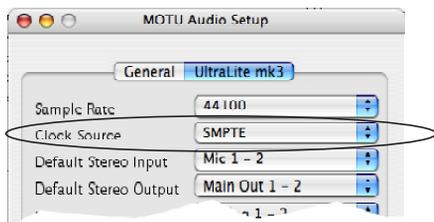
First, choose *SMPTE* as the clock source in AudioDesk, Digital Performer, or MOTU Audio Setup. This setting can also be made in the MOTU SMPTE Console (shown below).
