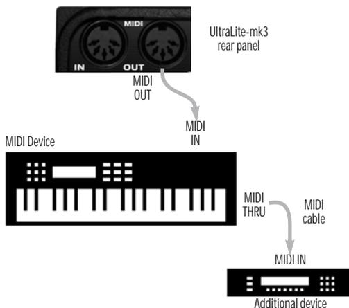
Figure 3-6: Connecting additional devices with MIDI THRU ports.
