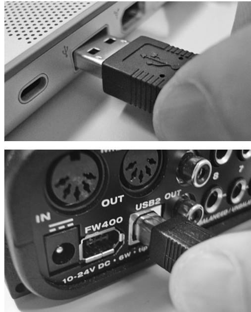
Figure 3-2: Connecting the UltraLite-mk3 to the computer via USB.
