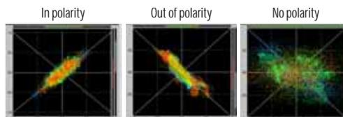
Figure 11-45: Checking polarity in a stereo signal with the X-Y Plot.
