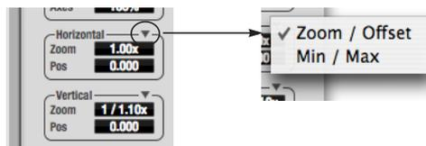
Figure 11-43: Setting the Horizontal or Vertical control modes.
