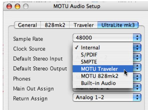
Figure 3-12: To resolve a MOTU FireWire interface to another Core Audio device, choose the other device from the Clock Source menu in MOTU Audio Setup. In this example, the UltraLite-mk3 will slave to the Traveler.
