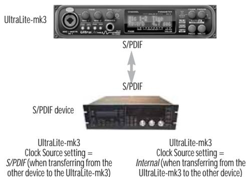
Figure 3-7: The setup for synchronizing a S/PDIF device with the UltraLite-mk3. Sync is achieved via the digital I/O connection itself. In this case, you have to choose S/PDIF as the UltraLite-mk3's clock source when recording from the other device.
