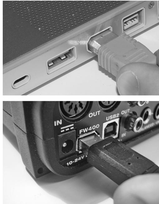
Figure 3-1: Connecting the UltraLite-mk3 to the computer via FireWire.
