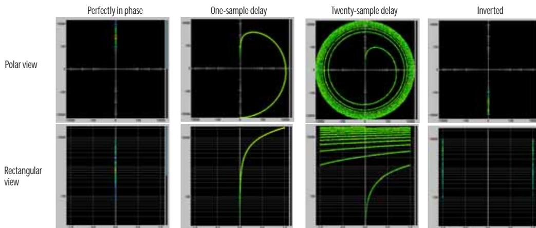
Figure 11-53: Two identical audio streams in the Phase Analysis.
