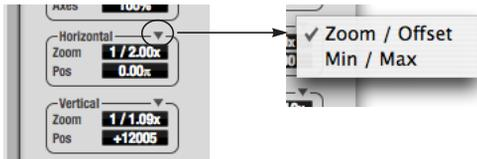
Figure 11-51: Setting the Horizontal or Vertical control modes.
