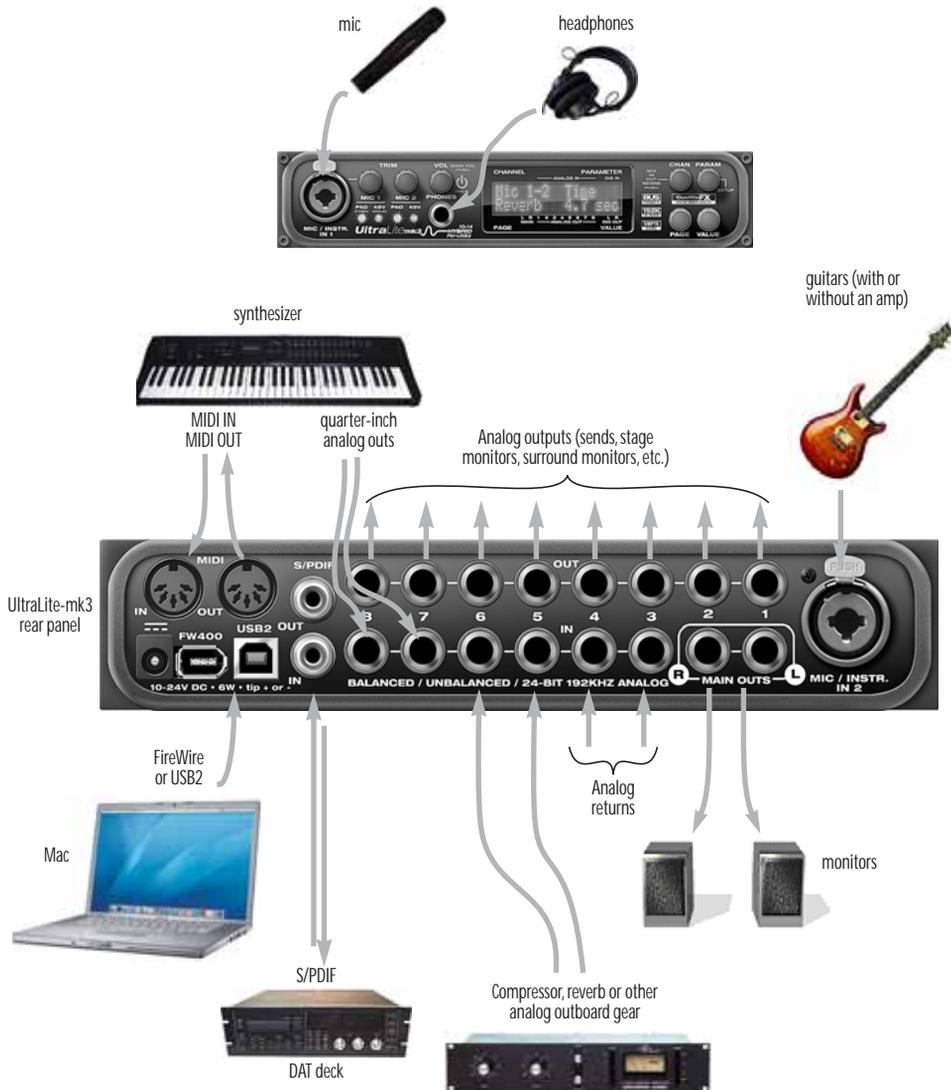
Figure 3-9: A typical UltraLite-mk3 studio setup.
