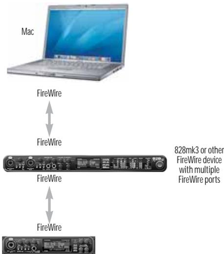
Figure 3-10: Connecting multiple MOTU FireWire audio interfaces.
