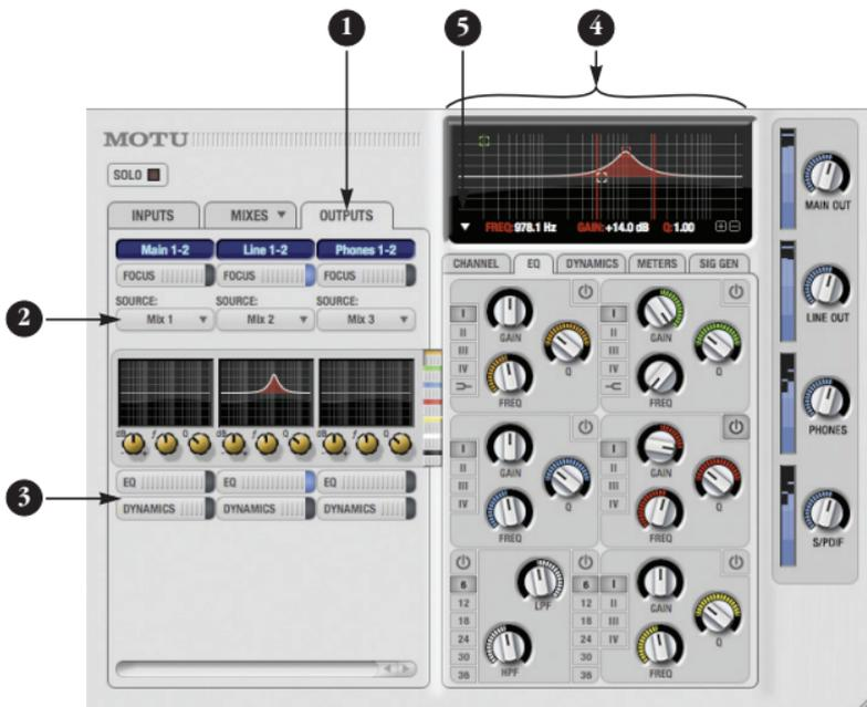
1. Click the Outputs tab to access settings for the MicroBook's outputs. For example, you can choose one of four different mixes for each output.
