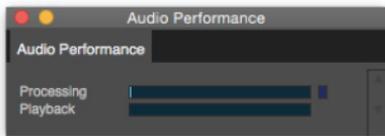
*Figure 5-7: When adjusting the buffer size to reduce monitoring latency, watch the 'Processing' meter in Digital Performer or AudioDesk's Performance Monitor. If you hear distortion, or if the Performance meter is peaking, try raising the buffer size.*
