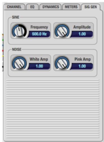
Figure 7-6: The Signal Generator tab.
