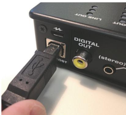
*Figure 4-4: Connecting the MicroBook to a computer.*
