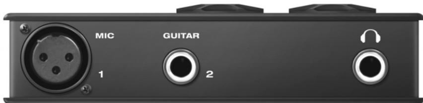
Do not use the stereo mini input and quarter-inch inputs at the same time. If you are using the mini jack, unplug the quarter-inch jacks. If you are using the quarter-inch jacks, unplug the mini jack.
