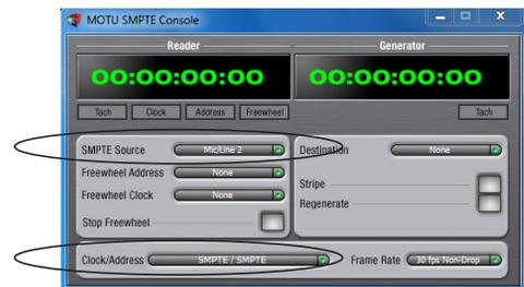
Launch the MOTU SMPTE Console and specify the *SMPTE Source*, which is the interface receiving the SMPTE time code. Also, confirm that the *Clock Source/Address* is *SMPTE/SMPTE*.
