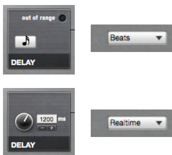
Figure 1-6: Choose real-time from the Tempo lock menu when you want to specify the delay time in milliseconds. Choose Beats, Note Values, or Bars to specify the delay time in musical values such as note duration or measure length. Beat and bar delay times stay locked to the tempo of your sequence, even through tempo changes.
