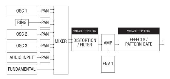
Figure 7-9: MX4 signal flow.
