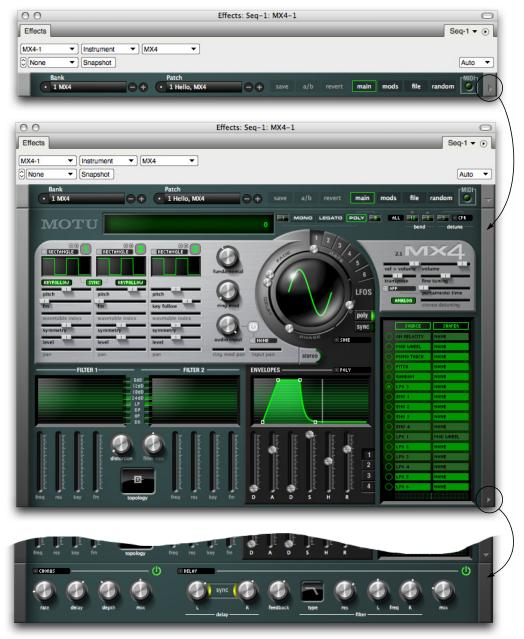
Figure 7-2: The Expand buttons.
