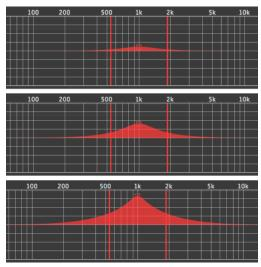
Figure 1-20: Type III EQ filter style.
