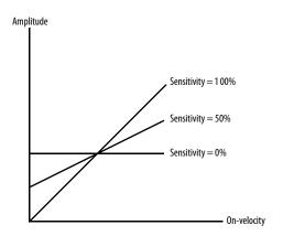
Figure 7-6: The affect of velocity sensitivity on sustain level.
