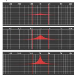
Figure 1-19: Type II EQ filter style.
